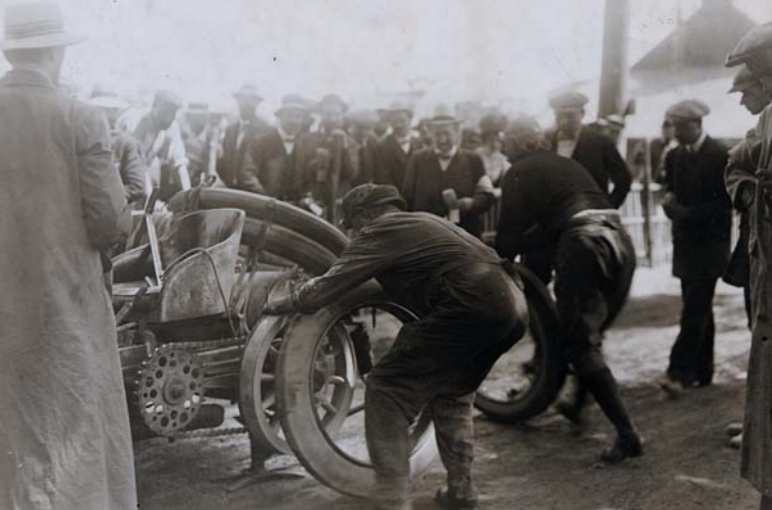
The detachable wheel rim. Collection A.C.O.
